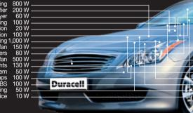
Stationary heating 800 W HIFI system, 4-channel amplifier 200 W Air conditioning 100 W Engine control/gnition 20 W Fuel injection 100 W Windscreen heating 1,000 W Passenger compartment fan 150 W Front windscreen wipers 80 W Radiator fan 500 W Headlight washing system 50 W EsP / ABS 100 W Steering wheel heating 50 W
