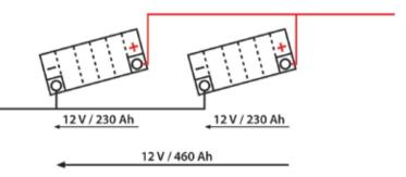
In a **parallel connection**, both the individual capacities and the cold start current of the individual batteries are combined.
