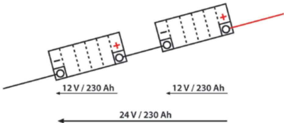
In the case of **serial connections** (=line connection) the voltages of the individual batteries are combined. Therefore, in order to create a 24V electrical system, two 12V batteries must be connected in series.
