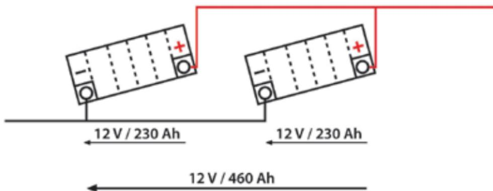
In a **parallel connection**, both the individual capacities and the cold start current of the individual batteries are combined.
