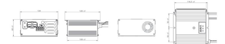
DIMENSIONS (LxWxH): 134x125x60 mm - 5.28x4.92x2.36 in WEIGHT: 1,20 Kg - 2.65 lbs PROTECTION GRADE IP30 INPUT VOLTAGE: Universal 100  $\div$  240 Vac – 50-60 Hz
