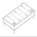
**Technology**Sealed AGM battery (electrolyte held in Absorbent Glass Mat separators) | dry-charged, acid pack is included | maintenance-free after initial filling
