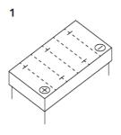
Sealed AGM battery (electrolyte held in Absorbent Glass Mat separators) | dry-charged, acid pack is included | maintenance-free after initial filling Technology
