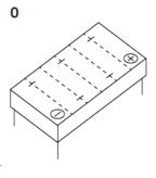
Sealed AGM battery (electrolyte held in Absorbent Glass Mat separators) | dry-charged, acid pack is included | maintenance-free after initial filling Technology
