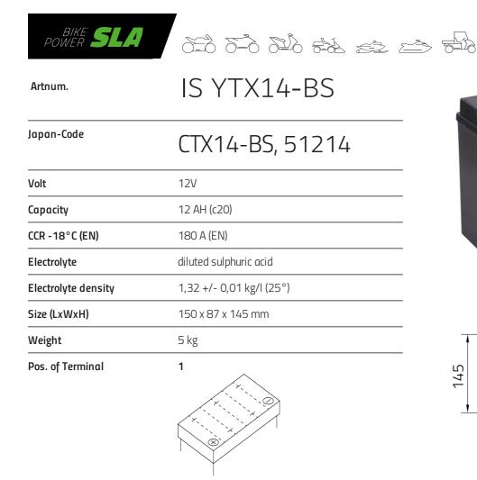
Sealed maintenance-free AGM battery (electrolyte held in Absorbent Glass Mat
