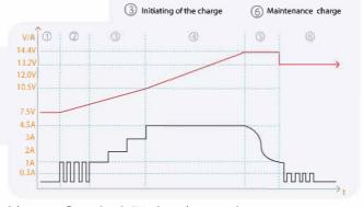
Pulse charge for battery reconditioning.
